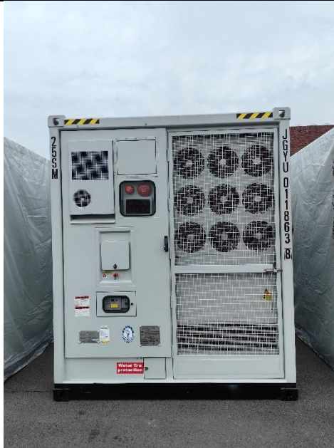
Side view with chiller and AUX power cabinet
